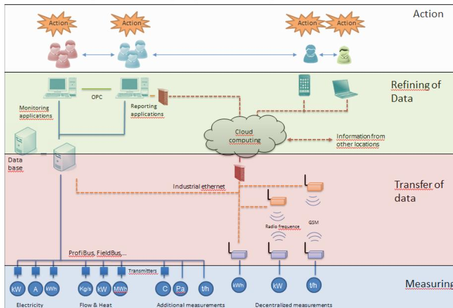
Figure 4. Simplified hierarchy of data transfer in process industry
